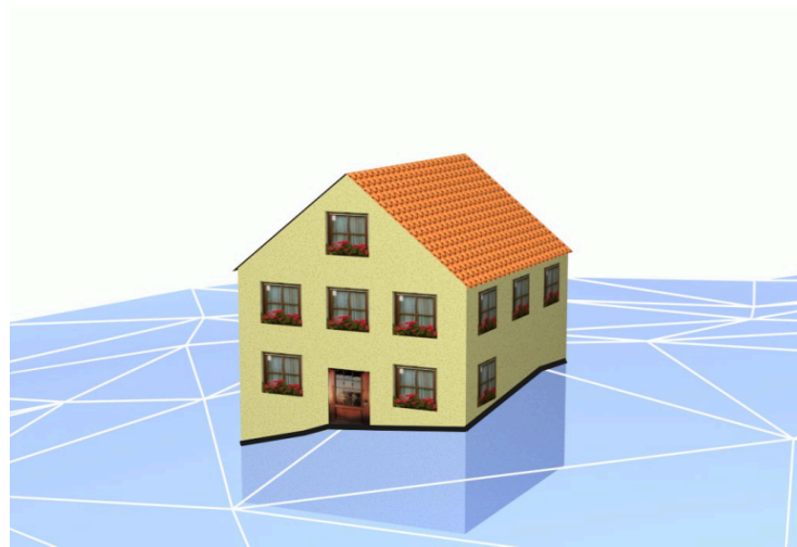
Figure 10-1 – TerrainIntersectionCurve for a building
