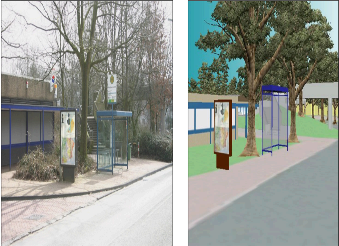
Figure 72 — Real situation showing a bus stop (left). The advertising billboard and the refuge are modelled as CityFurniture objects in the right image (source: 3D city model of Barkenberg).
