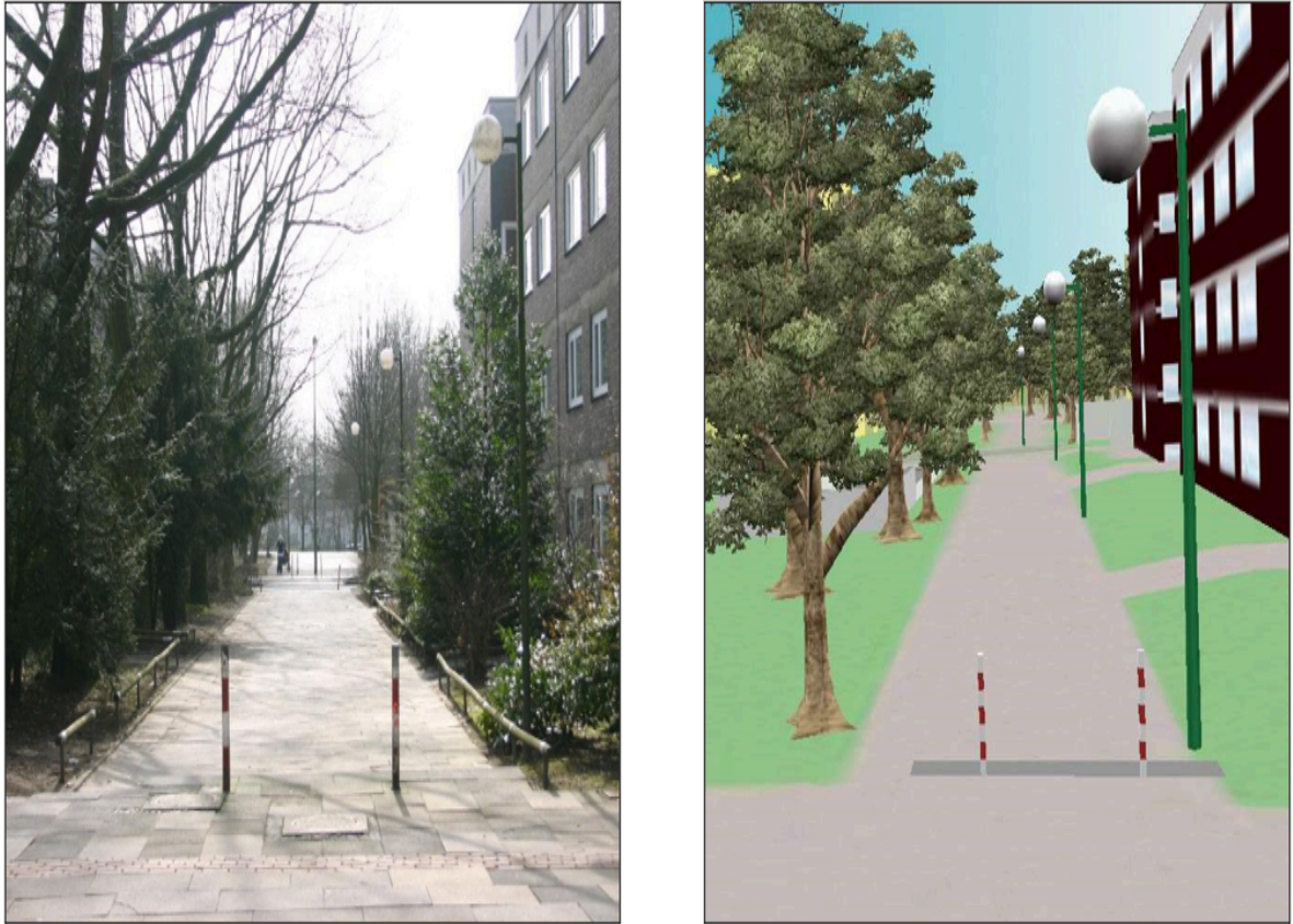
Figure 73 — Real situation showing lanterns and delimitation stakes (left). In the right image they are modelled as CityFurniture objects with ImplicitGeometry representations (source: 3D city model of Barkenberg).
