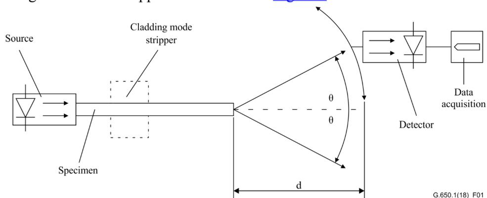
**Figure 1 — Typical arrangement of the far-field scan set-up**
