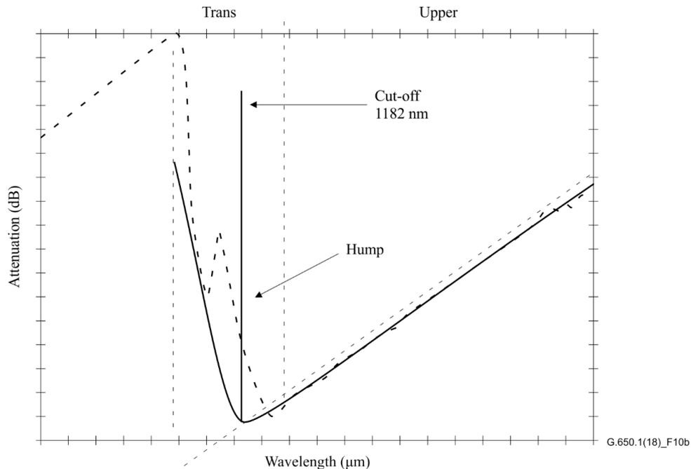
**Figure 10-b — Multimode reference cut-off plot with hump**
