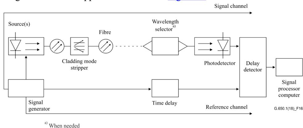
**Figure 16 — Typical arrangement of the test apparatus**
