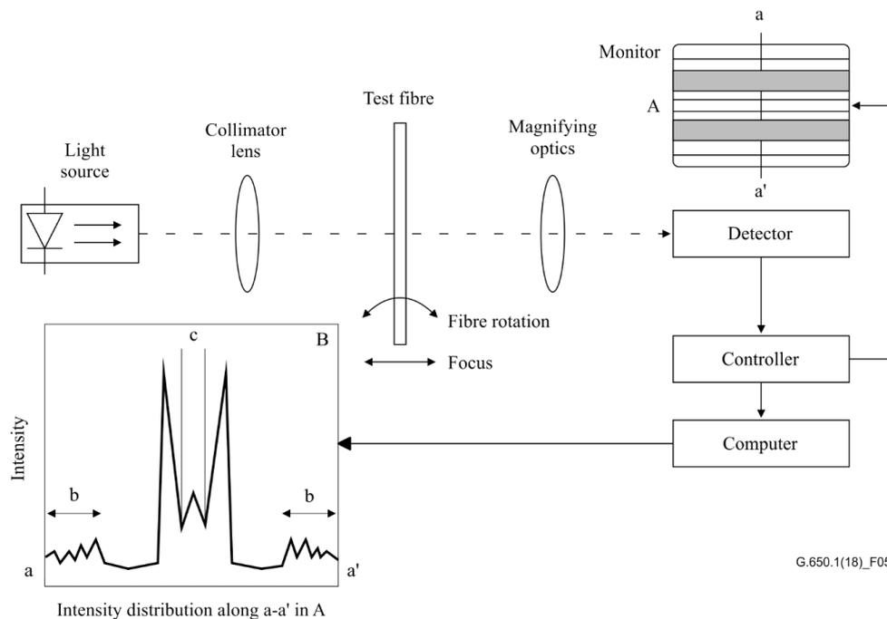
**Figure 5 — Schematic diagram of side-view measurement system**
