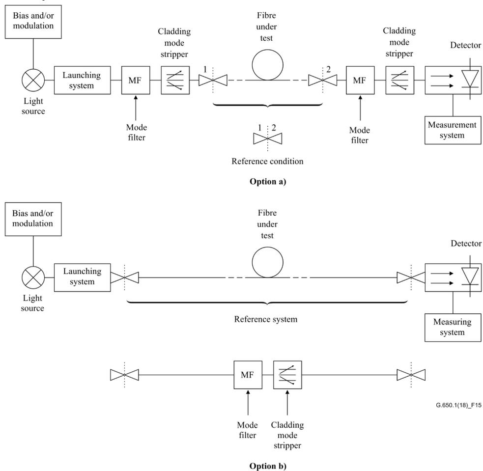
**Figure 15 — Typical arrangements for the insertion loss technique**
