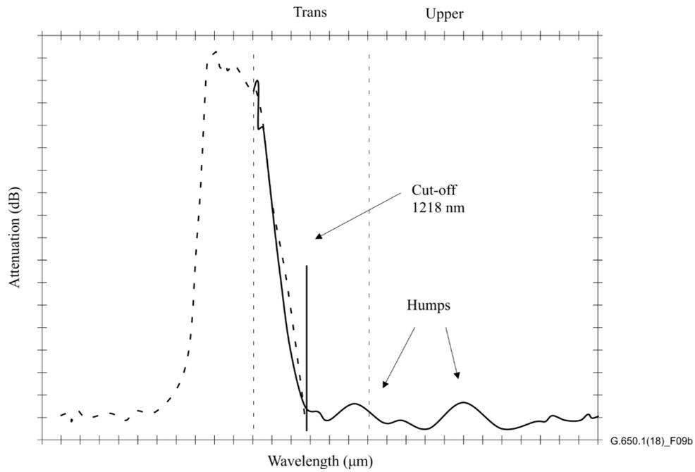
**Figure 9-b — Single-mode reference cut-off plot with humps**
