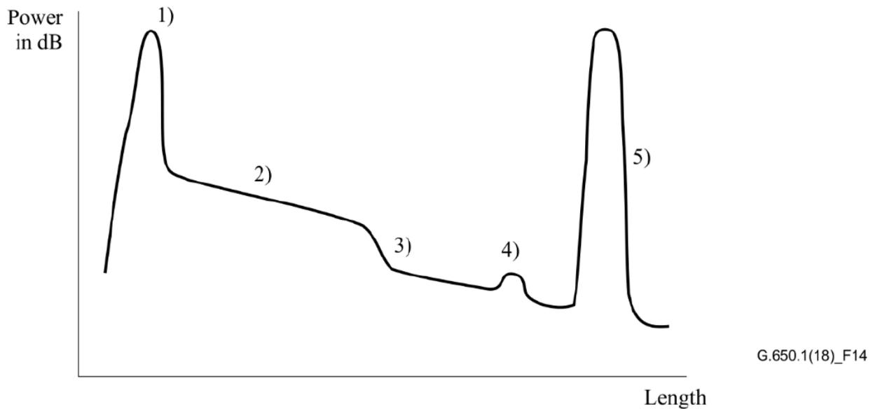
**Figure 14-b — Example of a unidirectional backscattering loss curve**
