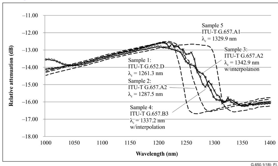
**Figure I.1 — Cut-off wavelength interpolation for some fibre samples**
