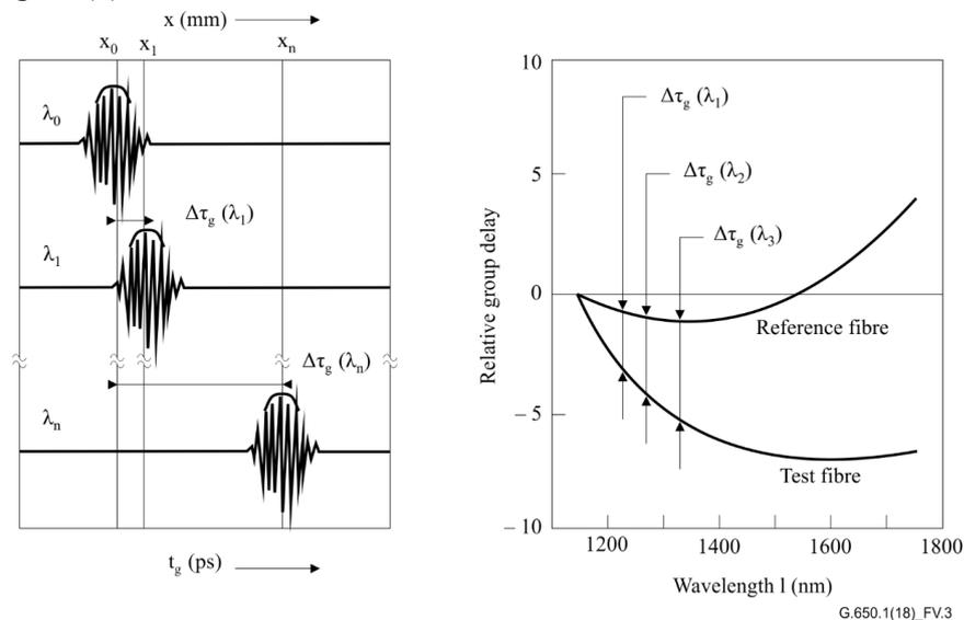
Figure V.3 — Determination of the spectral group delay
