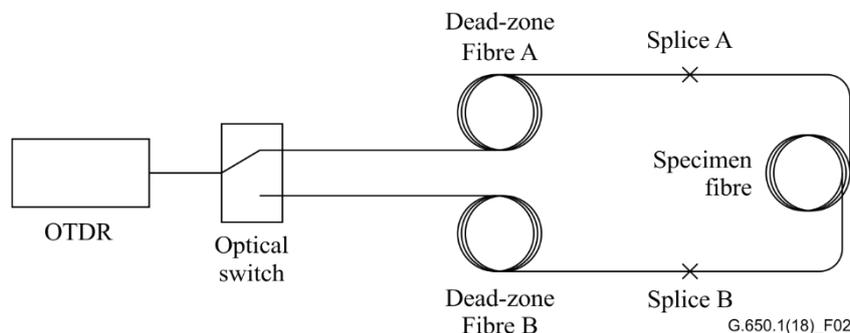
**Figure 2 — Optional apparatus for bidirectional backscatter**
