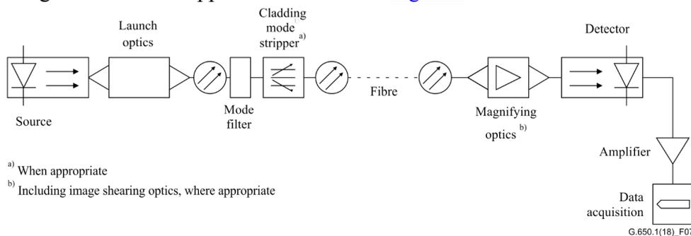
**Figure 7** — Typical arrangement of the transmitted near-field set-up
