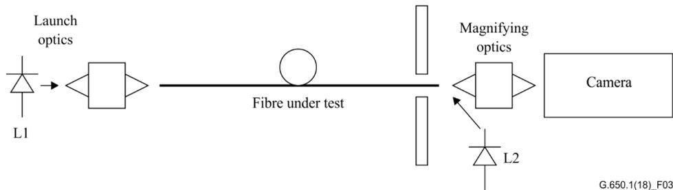
Figure 3 — A scheme for the test apparatus
